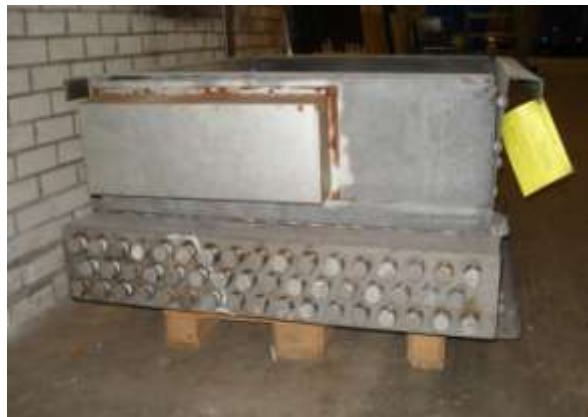
Figure 7a View from outside of bundle The 19 tubes are positioned on the left hand part
