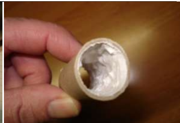
Figure B.2 Layer of gypsum paste
