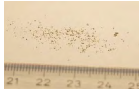
Figure 5: Result of a measurement showing a sub-threshold blockage in a good labelled tube.
