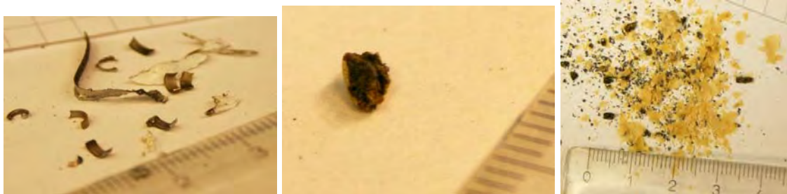
Figure 16: Non-specified flaws in group 3: Several chips, something like a small stone, paper-like dirt mixed with small chips.
