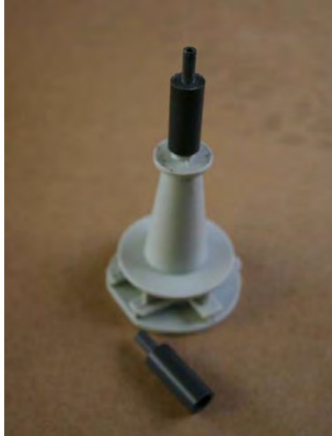
Figure 2: Turned adapter for tubes with inner diameter smaller than 8 mm.
