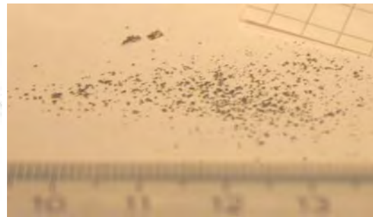
Figure 7: Indication of some particles spread over an elongated area inside the tube.
